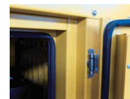
Double doors with double layer of rubber strip and heavy duty door lock
