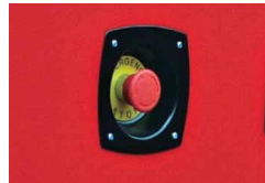
Emergency Stop Button Easy reachable on outside
